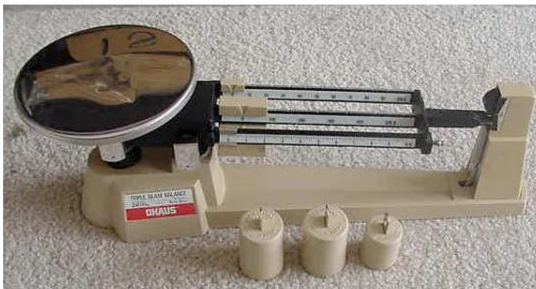
Figure 1-1. Photograph of an Ohaus Model 3600 Beam Balance. Courtesy of Ohaus Scale Corporation.
