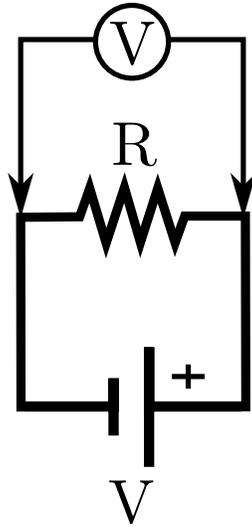
Figure 4: The simplest direct current circuit, with voltmeter installed.
