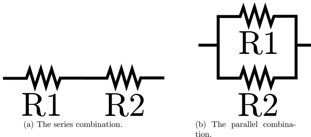
Figure 6: Series and parallel resistance combinations.
