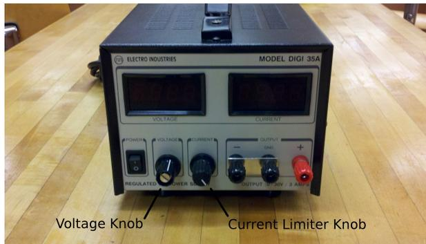
Figure 2: The direct current power supply.
